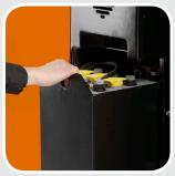
3. The design of the battery compartement allows easy access for maintenance purposes. The battery is mounted on rollers, which enables quick changing of the battery and supports multi-shift working.
